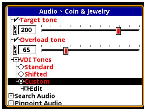
Selecting **Edit** pops up a small window which contains a list of VDIs, and each VDI has a slider for selecting a tone number from 0 to 255 (roughly 5 Hz to 1000 Hz):
