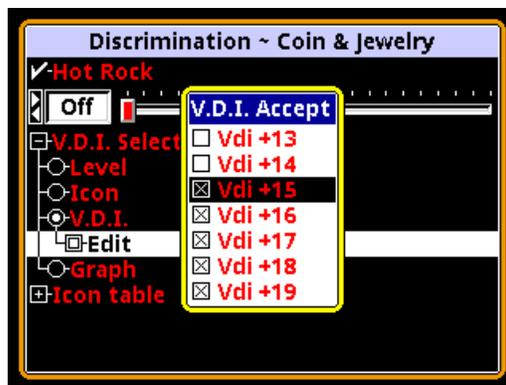
Selecting **VDI**→**Edit** pops up a small box which contains a list of VDIs, and each VDI has a checkbox next to it. This method is identical to the pop-up box on the Live Control Bar, already covered.
