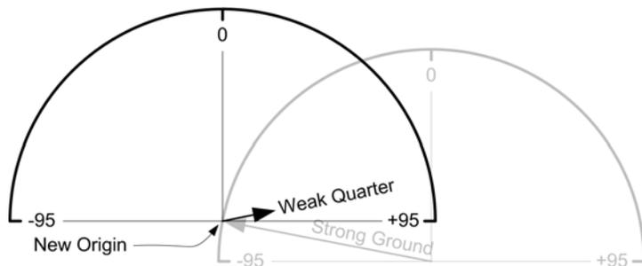
Any error in the ground balance point will result in an error in the target VDI response so it's important to maintain a decent ground balance point.
