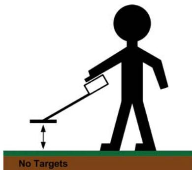
This manual ground balance sequence can be done at any time during normal search. Once the initial ground balance is completed, V3i will automatically track to most typical ground mineral changes.
